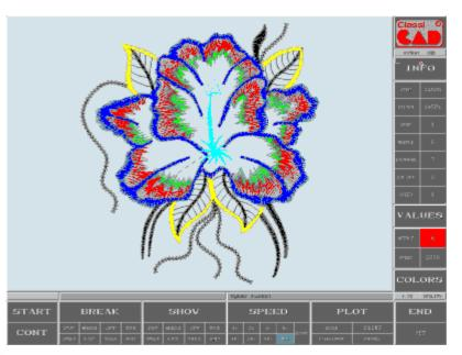
The computer screen images show the process of a CAD drawing that will eventually be used on a multi headed CAM embroidery machine
